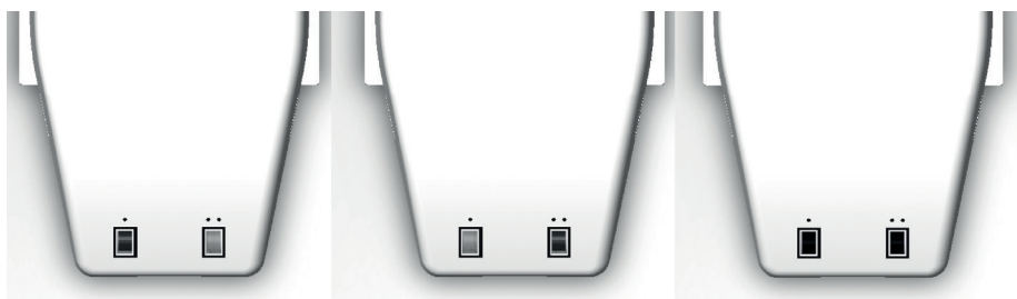
Figure 3: Infusion status indicator before activation (left), during infusion (centre) and after infusion (right).
